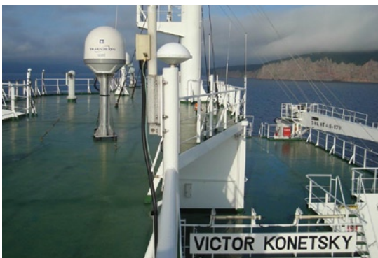
KVH's TracVision M9 provides satellite TV entertainment for crew members aboard many Unicom vessels, including the crude oil tanker Victor Konetsky.
