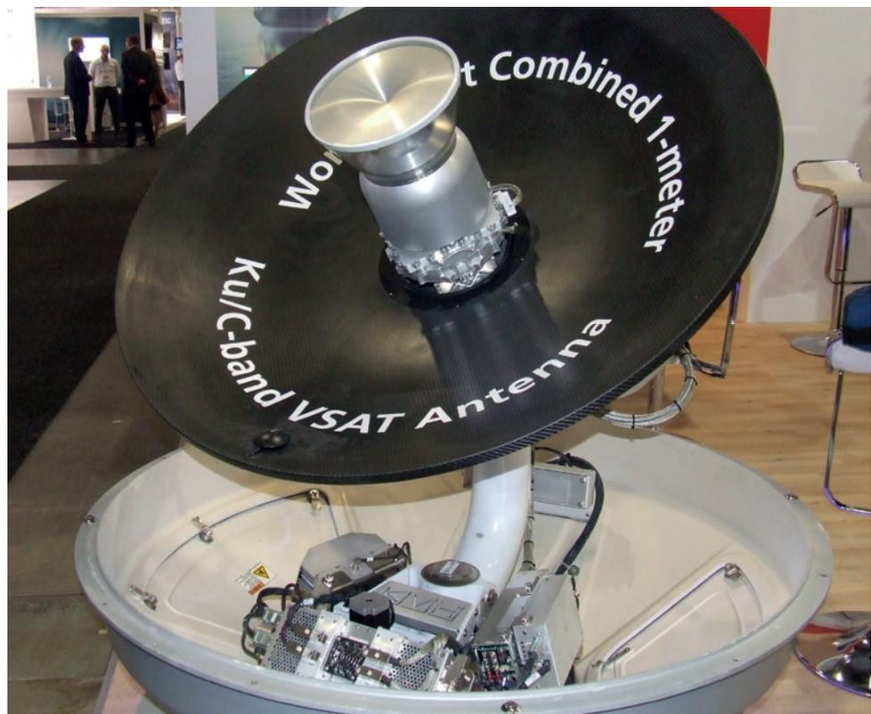
TracPhone V11-IP is a combined C-band and Ku-band antenna
