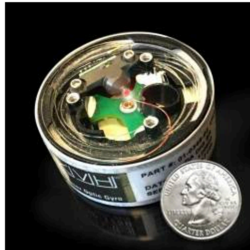
In this photo, the red illumination represents light moving through the FOG’s optical circuit of coiled fiber; this circuit is the FOG’s sensing unit and can be mounted with power and processing electronics within a driverless car to provide precise data for the car’s navigation systems. KVH photo ( Click image to enlarge. )
