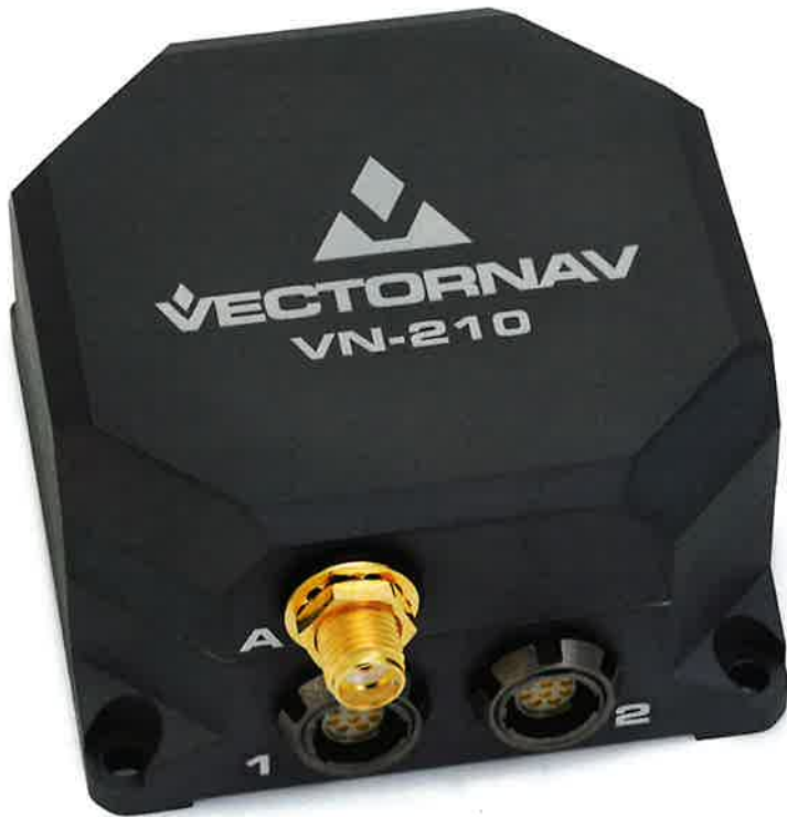
Coupling accelerometers, gyroscopes and GPS/GNSS data through an extended Kalman filter in an IMU provides position, velocity and attitude that can be orders of magnitude better than a standard navigation system (Courtesy of Vector Navigation)
